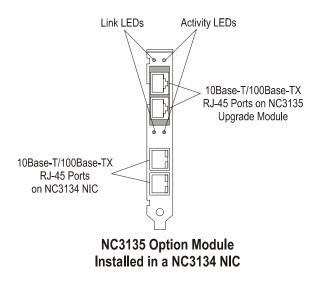
Figure 1-2. NC3135 Upgrade Module 10/100 ports and LED indicators
